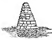
Fig. 10.—End view of half wall, on trench.
